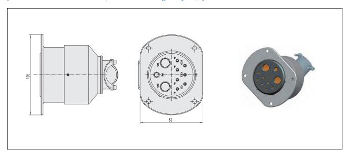
[BPC30-S-250A/750V-EV (vehicle mounting receptacle) ]
