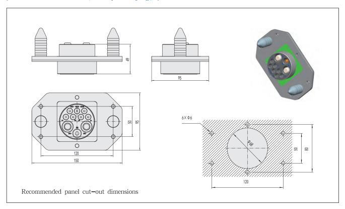
[BPC30-S-250A/750V-CR (bracket carrier receptacle)]
