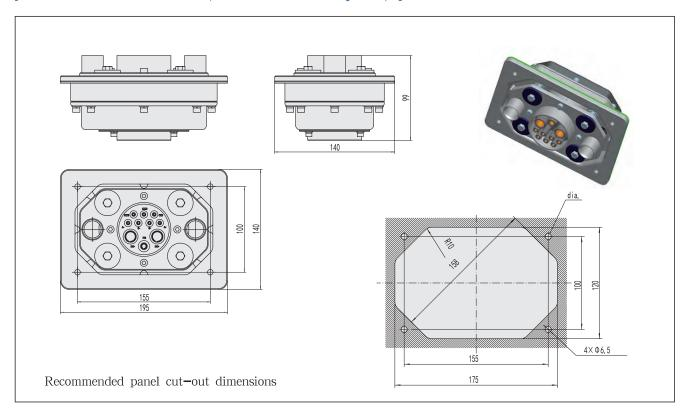
[BPC30-P-250A/750V-EV (vehicle mounting adapter)]
